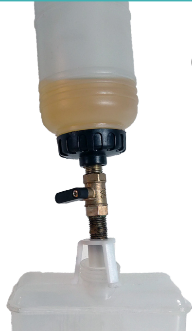
Photo 9: With any luck, you can use the filler reservoir, which makes the job a whole lot more convenient. You won't have to keep an eye on the level of the brake fluid reservoir.
