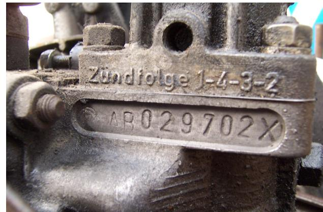
It is important to know which engine is installed when you want to order parts for that engine. Not every 1200 Split Bus has a 1200 cc engine. A lot of engines are interchangeable, often without modifications to the chassis or bodywork, so the odds are high that you have a different engine in the back of your car. Either a bigger displacement engine or an engine from another year.
