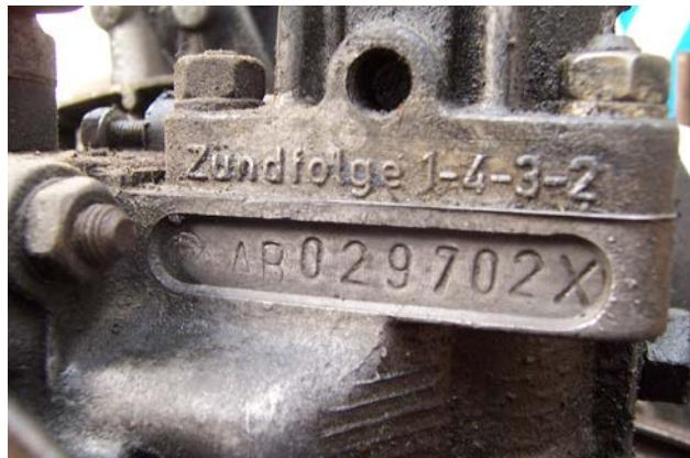
From the engine number you can determine what type of engine it is and the displacement of the engine.
