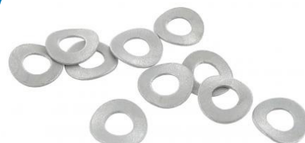
Curved M4 spring washers (10 pieces) Inner diameter: 4.3mm, Outer diameter: 9mm, Thickness: 0.5mm, Material: Galvanized steel
