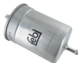
Fuel filter for injection engines Waterboxer engines 1900cc with engine code GW, Waterboxer engines 2100cc with engine code DJ, MV, SR or SS, hose connections: Ø 8mm
