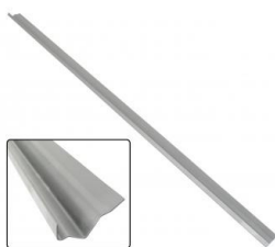
Roof gutter repair section Vanagon/T25 8.1984 and later
