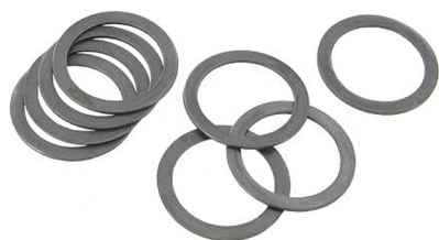
Rocker shaft shims for high-ratio rocker (8 pieces) for set #1780 and #1781, Thickness: 0.381mm, Inner size: 19.50mm, Outer size: 25.40mm
