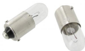
Sidelight, turn indicator, interior- and license plate lighting bulb 12V clear (per pair) Type: bayonet, Base: BA9s, Color: clear, voltsage: 12V, Power: 4 Watt
