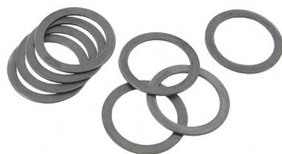
Rocker shaft shims for high-ratio rocker kit #1780 and #1781 (8 pieces) Thickness: 0.254mm, Inner size: 19.50mm, Outer size: 25.40mm
