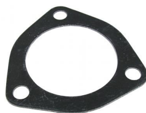
Exhaust header to muffler gasket (each) Bolt distance: 78mm, Inner size: 68mm
