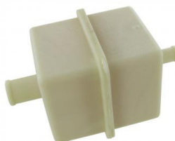
Fuel filter for injection engines Type-1 engines until 1.1980, Type-3 engines, Type-4 engines 8.1974 and later, Waterboxer engines with engine code DH, hose connections: Ø 8 and Ø 12mm
