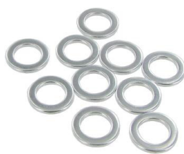
7 mm washers 12 mm wide (10 pieces) Inner diameter: 7mm, Outer diameter: 12mm, Thickness: 1.2mm, Material: Galvanized steel, Hardness: 200 HV
