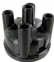
Distributor cap A-quality Type-1 engines 30hp 8.1960 and later, 34hp until 7.1965, 1200cc, 1300cc and 1500cc until 7.1968, 1600cc until 7.1970, Type-3 engines 1500cc 8.1963 until 7.1968, 1600cc all years
