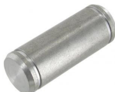
Handbrake bearing pin Beetle export models, VW 1300, VW 1500, 1302, 1303 and convertibles 8.1955 and later, Beetle standard models and VW 1200 1962 (VIN 4 630 938) and later, Karmann Ghia all models and years, Type 3 all models and years, Thing all models and years
