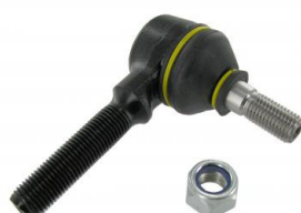
Tie rod end A-quality Beetle 1968 (VIN 118 857 240) and later, Karmann Ghia 1968 (VIN 148 857 240) and later, Bus 8.1967 until 7.1979, Type 3 8.1967 and later, Thing
