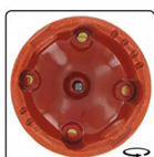
Distributor cap B-quality Type-1 engines 30hp 8.1960 and later, 34hp until 7.1965, 1200cc, 1300cc and 1500cc until 7.1968, 1600cc until 7.1970, Type-3 engines 1500cc 8.1963 until 7.1968, 1600cc all years
