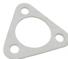
Exhaust header to muffler gasket (each) Bolt distance: 58mm, Inner size: 44.70mm
