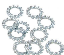
External serrated lock washers M6 (10 pieces) Inner diameter: 6,4mm, Outer diameter: 11mm, Height: 2.1mm, Material: Galvanized steel
