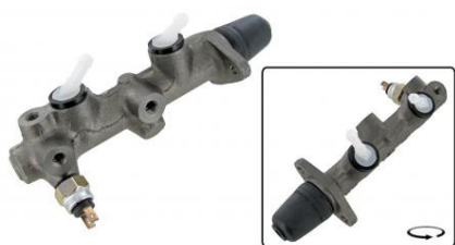
Master brake cylinder split braking system without brake warning light Beetle VW1200, VW1300 and VW1500 LHD, Karmann Ghia LHD, Thing LHD
