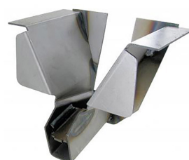
Rear jacking point (each) Bus until 7.1967
