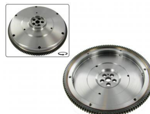
215 mm conversion flywheel Type-4 engines
