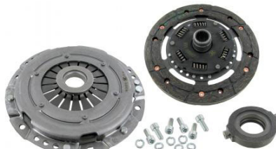
Clutch kit 180 mm Type-1 engines 25hp+30hp, 1200cc until 1972 (VIN 112 2670 582), 1300cc until 7.1970, Type-3 engines until 7.1962
