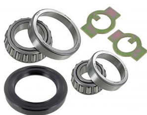
Front wheel bearing kit one side Bus 8.1963 until 7.1967
