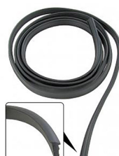
Easyfit pop-out seal between frame and glass (each) Bus until 7.1967
