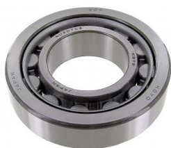
Outer rear wheel bearing (each) Bus 8.1963 until 7.1970
