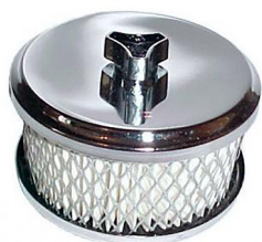
Chrome mini air cleaner Ø100 mm height 60 mm (each) Solex stock carburetors (51mm neck)
