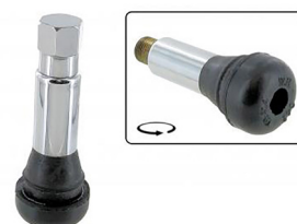
Chrome-plated stock valve stem (each) Mounting hole: 11.5mm, Height: 43mm
