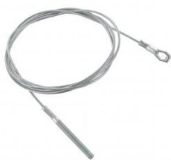
Clutch inner cable Type 3 1965 (VIN 315 125 561) and later
