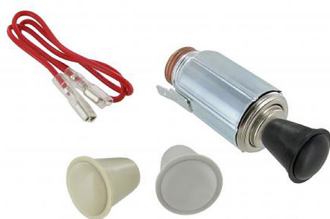
Cigarette lighter with 3 color knobs voltsage: 6V-12V, Mounting hole: 22-25mm, Board thickness: maximum 8mm
