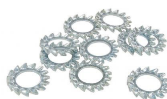
External serrated lock washers M8 (10 pieces) Inner diameter: 8,4mm, Outer diameter: 15mm, Height: 2.4mm, Material: Galvanized steel
