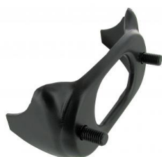
Transmission mount bracket front Beetle 8.1960 until 7.1972 and 1.1986 and later, Karmann Ghia 8.1960 until 7.1972, Thing
