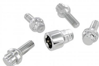
Wheel locks for bolts with convex collar (4 pieces) Thread size: M12 X 1.5, Total length: 50mm, Thread length: 25mm, Wrench size: 17 and 19mm, Collar: ball
