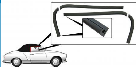
Door seal around door glass left and right (4-part) Karmann Ghia convertible
