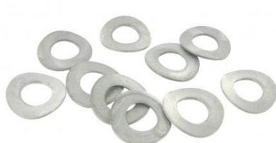
Curved M10 spring washers (10 pieces) Inner diameter: 10.5mm, Outer diameter: 21mm, Thickness: 1.0mm, Material: Galvanized steel
