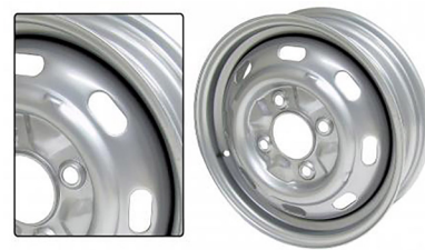
Standard wheel grey (each) PCD: 4 x 130mm, Size: 4.5 x 15 inch, ET: +45mm
