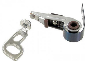
Ignition points Type-1 engines 25hp, 30hp until 12.1960
