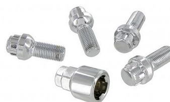
Chrome wheel lock bolts (4 pieces) Thread size: M14 X 1.5, Total length: 50mm, Thread length: 25mm, Wrench size: 17 and 19mm, Collar: ball
