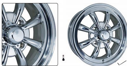
EMPI GT-8 wheel polished (each) PCD: 4 x 130mm, Size: 5.5 x 15 inch, ET: +30mm, Backspacing: 4 3/8 inch
