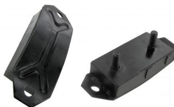
Transmission/engine mount rear (per pair) Beetle until 7.1972 and 1.1986 and later, Karmann Ghia until 7.1972, Bus until 7.1967, Type 3, Thing
