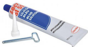
SI 5926 blue silicone sealing compound Content: 100 ml, Color: blue, Chemical Type: Acetoxy Silicone, Maximum sealing gap: 1.0mm, Temperature range: -54 °C to +150 °C
