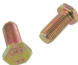
Seat belt bolts (per pair) Thread size: 7/16 UNF, Length: 25mm, Hardness: 8.8, Material: galvanized steel, Wrench size: 17mm
