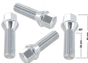
Wheel bolts chromed (4 pieces) Thread size: M14 X 1.5, Total length: 64mm, Thread length: 38mm, Wrench size: 17mm, Collar: 60°
