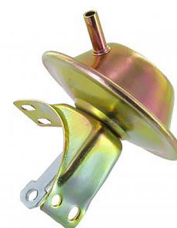
Distributor vacuum advance Type-1 engines 1200 D 1974 (1 268 063) until 1975 (1 357 043), 1300 AC 1973 (0 07 320) and later, AB 1973 (830 938) and later, AR all years, 1600 AF 1972 (032 051) and later, AD 1973 (754 528) and later, AS all years, AL until 8.1975, CT engines all
