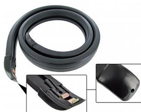
Rear bumper rubber impact strip Bus 8.1972 until 7.1979
