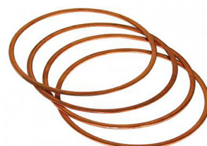
Copper cylinder head spacers (4 pieces) Type-1 engines, Type-3 engines, CT/CZ engines, Thickness: 1.016mm, Outer diameter: 101mm, Bore: 94.0mm, Material: copper
