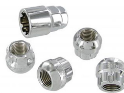
Chrome wheel lock nuts (4 pieces) Thread size: M14 x 1.5, Height: 21mm, Wrench size: 19 and 21mm, Collar: ball
