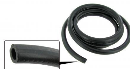
Fuel hose textile braided (per meter) Inner diameter: 8.00 (max. 8.50mm), Outer diameter: 13.70 (max. 14.20mm), Working pressure: 7.5 bar, Bursting pressure: 30 bar
