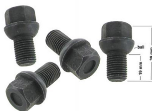
Wheel bolts black oxide (stock bolt) (4 pieces) Thread size: M14 X 1.5, Total length: 39mm, Thread length: 19mm, Wrench size: 19mm, Collar: ball
