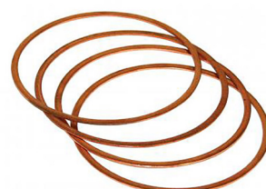
Copper cylinder head spacers (4 pieces) Type-1 engines, Type-3 engines, CT/CZ engines, Thickness: 1.016mm, Outer diameter: 98mm, Bore: 90.5 and 92.0mm, Material: copper
