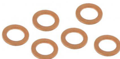
Sealing rings M6 (6 pieces) Inner diameter: 6mm, Outer diameter: 10mm, Thickness: 1mm, Material: copper
