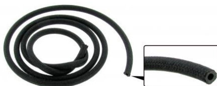
Fuel hose with a textile outside (per meter) Inner diameter: 5.0mm, Outer diameter: 9.5mm, Working pressure: 7 bar, Bursting pressure: 30 bar
