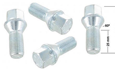
Wheel bolts galvanized (4 pieces) Thread size: M14 X 1.5, Total length: 48mm, Thread length: 25mm, Wrench size: 17mm, Collar: 60°
