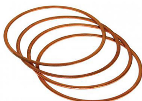
Copper cylinder head spacers (4 pieces) Type-1 engines, Type-3 engines, CT/CZ engines, Thickness: 1.27mm, Outer diameter: 98mm, Bore: 90.5 and 92.0mm, Material: copper
