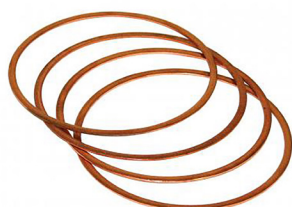
Copper cylinder head spacers (4 pieces) Type-1 engines, Type-3 engines, CT/CZ engines, Thickness: 1.524mm, Outer diameter: 98mm, Bore: 90.5 and 92.0mm, Material: copper
