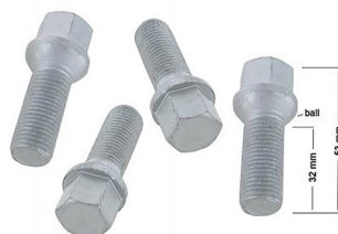
Wheel bolts galvanized (4 pieces) Thread size: M14 X 1.5, Total length: 53mm, Thread length: 32mm, Wrench size: 17mm, Collar: ball
