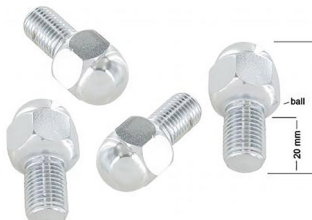
Wheel bolts chromed (4 pieces) Thread size: M14 X 1.5, Total length: 45mm, Thread length: 20mm, Wrench size: 22mm, Collar: ball
