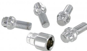
Chrome wheel lock bolts (4 pieces) Thread size: M14 X 1.5, Total length: 50mm, Thread length: 25mm, Wrench size: 17 and 19mm, Collar: ball
