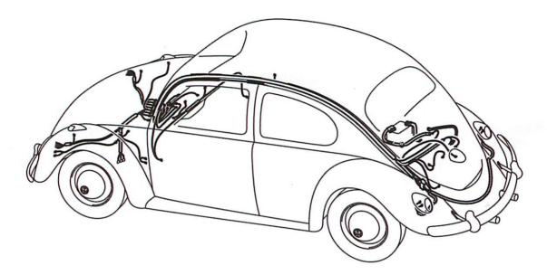
1961 Bug Wiring Harness Kit. This wiring harness kit fits 6-volt and 12-volt 1961 Bug sedan models. If your Bug has electrical upgrades, such as an alternator, or additional equipment, some modifications will be required.
