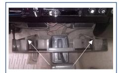
Two clips, one either side need to be pressed down with a flat head screw.
