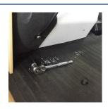
Remove the bolt for the seat belt, this allows you to remove any original seat box carpet.
