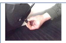
Removes the seat belt anchorage plastic to gain access to the bolt.
