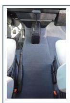
Once the hole for the handbrake has been cut, line up the front of the walkthrough carpet with the seat boxes and glue into place.
