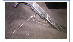
The throttle linkage can now be removed by pulling the pedal upwards.
