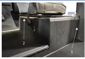
Start by spray gluing the back of the carpet and the seat box also. Start at point number one and work the carpet around the box. You will notice a fibreboard piece along the top of the carpet, this will need to be turned down and into the body (point number two).
