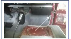
Pinpoint any fixing that would have been removed from the original carpet and then make the incisions ready for the clips to be reused and refitted.
