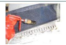
Then glue the back of the wheel arch carpet along the binded edge.
