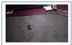
The next item to remove is the plastic studs that hold the carpet fixings on the bulkhead. A flat head screwdriver can be used.
