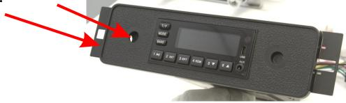
Step Three: Remove the faceplate and check the trace marks, then use tin snips to cut off the edges of the Infinimount Bracket and use a drill to drill out the traced holes for the shafts to fit through. Remount the Infinimount Brackets in the standard 4 hole position
