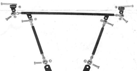
Requires that a 2" hole (approx) be drilled in both wheel wells to allow the Cross Truss Bar End Links to come thru the apron and bolt to the upper shock tower (except 67-68).
