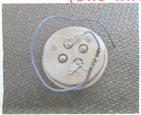
1. The backside of Horn button, the blue wire is the ground
