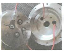
3. The two cables is connected to the pin seperately
