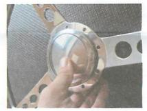
4. Test it working good, lubricate O-ring before Pushing down to the steering wheel
