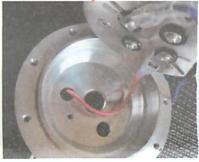
2. Connecting the positive cable from the column or adapter to positive pin
