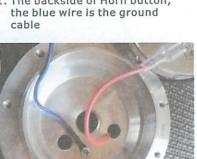
3. Ground the blue wire using self-tapping screw on the adapter
