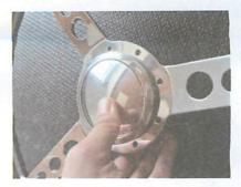
4. Test it working good, lubricate O-ring before Pushing down to the steering wheel
