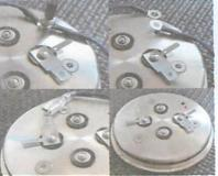
2. Unscrew and unplug, remove blue wire at back of horn button
