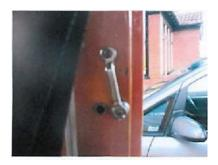
**Step 4:** Attach the bracket and spacer using the 2 cm screw to hold the spacer in place. Repeat the bracket installation on the other B pillar. Check all screws are tight.
