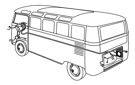
1964 Bus Export Model Wiring Harness Kit. This wiring harness kit fits 6-volt and 12-volt U.S. export Bus models. This model has an 8-fuse push-on terminal fuse box.
