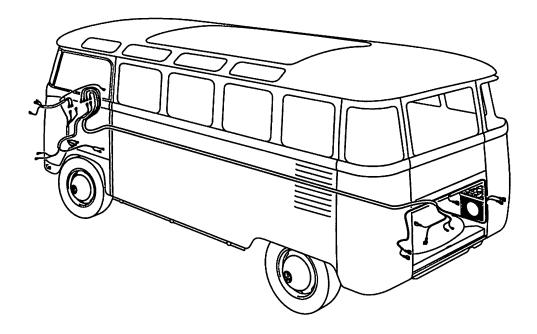
Mid'60-1963 Bus Export Model Wiring Harness Kit This wiring harness kit fits 6-volt and 12-volt U.S. export Bus models from Mid'60 (starting at VIN # 614456) – 1963 Bus. These models have an 8-fuse push-on terminal fuse box. This will also work with 1960 Bus models between VIN #'s 569929-614455, however the push-on terminals will need to be removed as these models have screw terminal connections.
