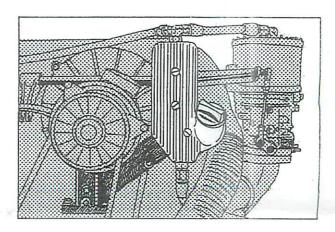
With the standard oil filler and vent tube removed, clean the top of the oil tower surface and threads. Place a small amount of engine sealer or silicone around the mating surfaces between the generator oil tower and your Oil Filler Breather Box. Install and tighten the oil tower gland nut. The nut must be torqued to at least 20 lbs.
