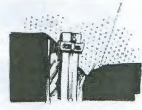
13. The handstrap mounting bracket holds this folded edge snugly against the door post upholstery and provides a pleasant finishing touch.
