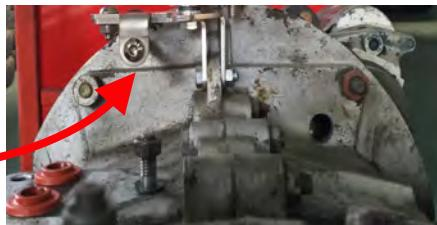
3. Install the top pulley. There are 2 spacer, the flat goes to the lower of base, and the corn goes between the base and the pulley.
