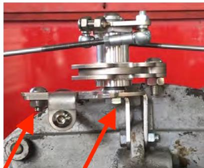
4. Make sure the STOPPER is at the front of the base, see photos, then tighten the 3xM8 as arrow.
