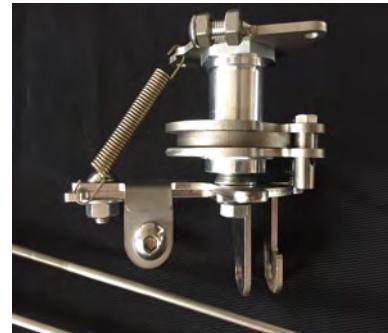
7. Install the pushing plate on the carbs (left and right)
