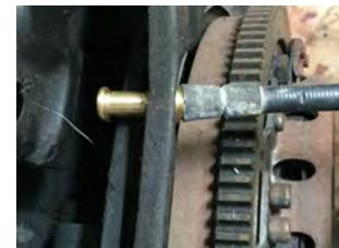
10. Install the accelerator cable.
