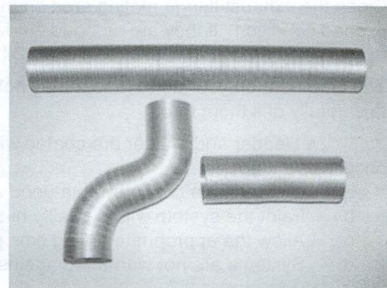
Cut the Heater Hose included with your header in half. Then bend the tubing to fit from the fan housing around the upper header pipe and down to the heater box.
