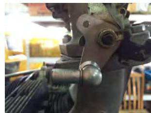
8. Install the linkage arms, cut the arm to desire length for left side and right side.
