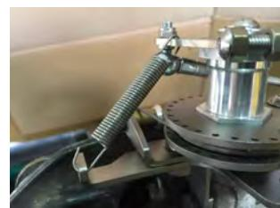
7. Install the pushing plate on the carbs (left and right)
