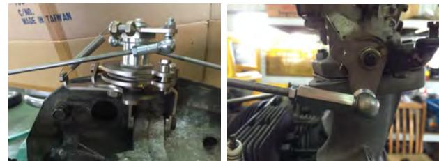
9. Install the accelerator cable.
