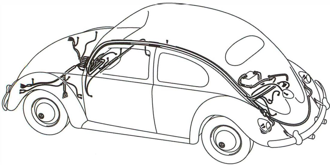
1956-1957 Bug Wiring Harness Kit. This wiring harness kit fits 6-volt and 12-volt 1956-1957 Bug sedan models. If your Bug has electrical upgrades, such as an alternator, or additional equipment, some modifications will be required.
