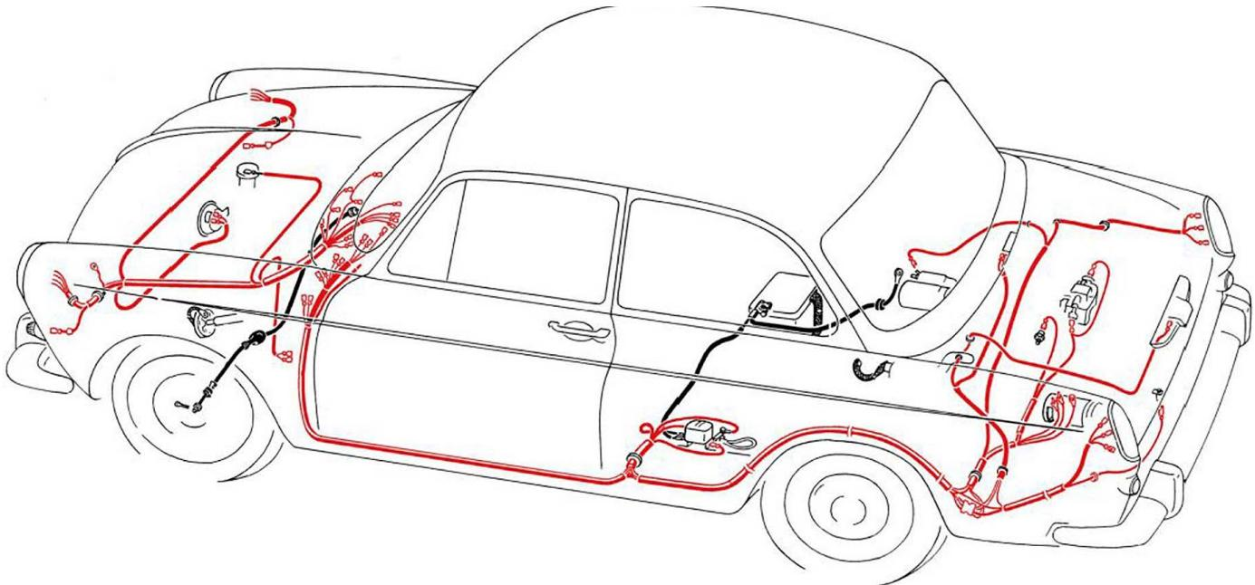
New Type 3 wiring harness fitting U.S. Spec. 1961-1969 carbureted Type 3 models. This wiring harness works with 6-volt and 12-volt electrical systems. If your Type 3 is a European model, or has had some electrical "upgrades" done to it, some modifications will be required. This wiring harness includes the major components; some miscellaneous wires will be required.
