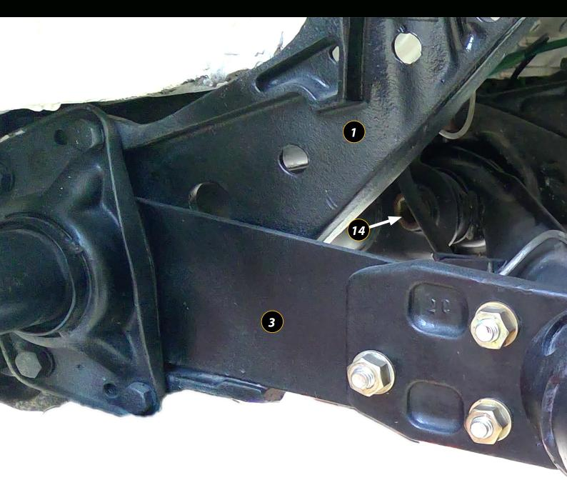
This picture shows the IRS drive of a VW 1303. All the parts we showed earlier in the drawing are now shown in practice. In the next editions we will disassemble and overhaul both the swing axle and the IRS in detail.
