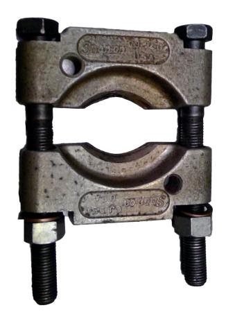
When the parts are mounted very close together, as can be seen on the picture on the next page, this back puller come in handy (picture at the top). The photos show how to remove the bearing from an alternator rotor (photo at the top of page 32) without damaging the shaft. The photo at the bottom of page 32 shows the same tool used for the dynamo bearing.
