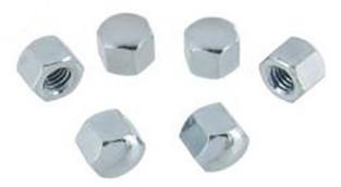
The correct way to tighten these M6 nuts is with a small torque wrench. The cap nuts of the Volkswagen Type 1 engine are tightened with 7 Nm (0.7 kgm), that's not much at all. You can also tighten the cap nuts on the feel, but beware, 7 Nm you have reached very quickly with a ratchet arm of 20 cm.
