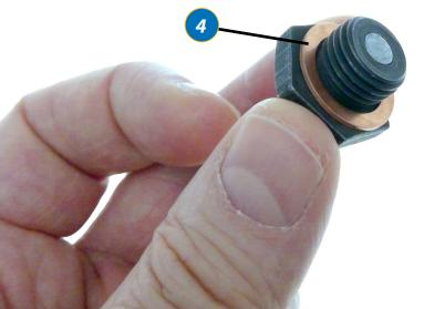
Six M6 copper packing rings (number 6) and one M14 (number 4) copper packing ring are used to make the sump plate of the Type 1 engine leak free.
