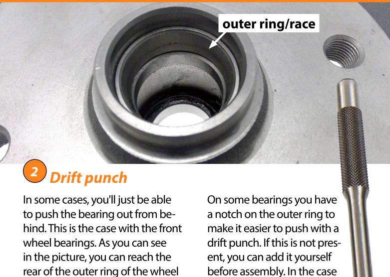
It is of course always recommended to warm up the drum to make it easier to remove the bearing. The tension will drop considerably by increasing the temperature.
