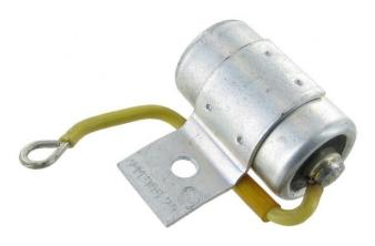
How do you measure if a condenser is working or not? A condenser is not just an electrical resistor. You sometimes hear that a resistance meter (ohmmeter) is used to know if the condenser is still working. But a resistance meter will only tell you if the insulation (dielectric, see edition 18 page 17) inside the condenser is in a short circuit, in other words it is burnt out, nothing more.
