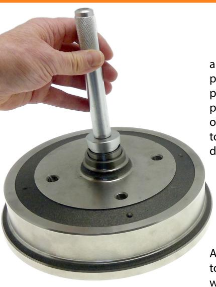
area. The bearing drive must be placed vertically, axially, perpendicular to the bearing. If you position the bearing drive too obliquely, the bearing tends to go in at an angle, which can damage the part.
