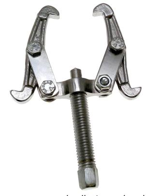
Above: an external puller is very handy but you need to have the necessary space to grab behind the bearing.
