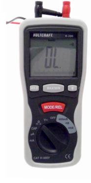
Measuring a condenser with a resistor meter only gives a usable result in one case, namely when the resistor is zero, the condenser needs to be replaced. In the second case, you don't know what to do with the condenser.
