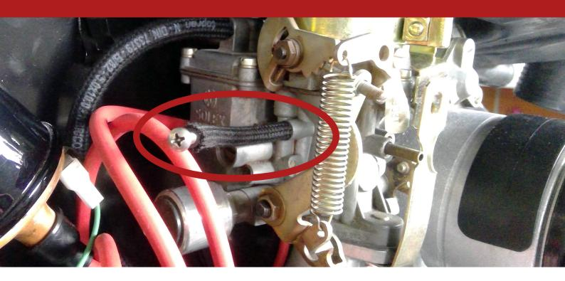
The vacuum hose has to be disconnected on some engines with vacuum advance (refer to the original Volkswagen workshop manual: Bentley series). We show a partial table on page 42.
