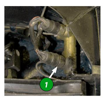
We show the master brake cylinder of the VW 1303 below. You can see the two connections for the brake lines, one line to activate the front wheels and one line for the rear wheels. The connection with the brake pedal rod is hidden under the rubber dust cap. A dual brake circuit is of course safer than a single circuit, if one circuit fails you always have two wheels with brake power left. Two brake light switches (2) are installed on this type of master brake cylinder.
