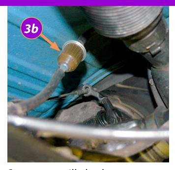
Some cars will also have an extra fuel filter (3b), it is most of the time installed underneath the car as shown in the picture above (3b) and on the drawing on page 29 (3b). Check if this filter is not clogged and if it is correctly installed, most fuel filters have an input and output.
