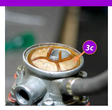
The fuel will also be filtered in the fuel pump. There is an extra filter built into the pump (3c) as shown on the picture above.
