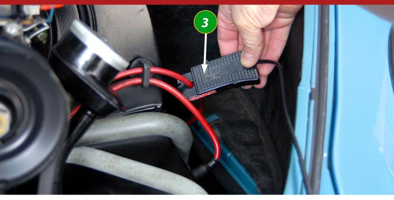
The induction clamp is now installed on the spark plug cable of cylinder 1 as showed on the picture above (why cylinder 1? we explained that in edition 14). The induction clamp should be installed as indicated in your manual, most clamps have a sign printed or painted to show which side should point towards the spark plug.
