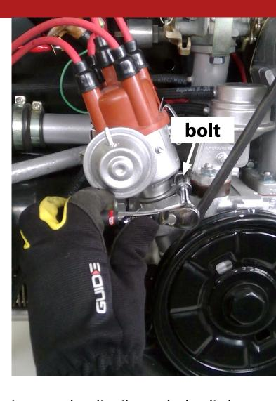
We show on the picture above (sourced from an old VW workshop manual) how to position the strobe light. The 7,5° mark on the crankshaft pulley should be in line with the center of the crankcase, where both crankcase halves meet. If not, you will need to rotate the distributor clockwise or counterclockwise to tune the ignition timing.
