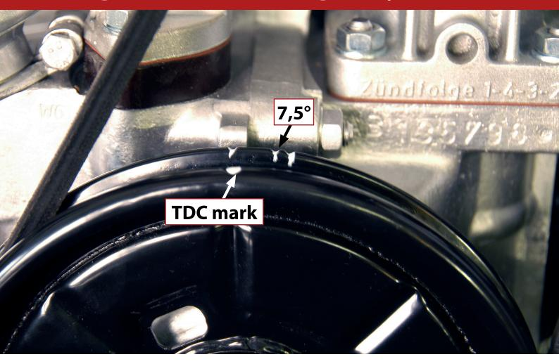
The distributor and the crank-shaft pulley on our AB engine are not original. The distributor has only one vacuum hose, so we need to set the ignition timing at 7,5° before the TDC (ignition advance) and not 5° after TDC as mentioned in the workshop manual. Ask a VW professional for advice if you are not sure about the ignition timing value.
