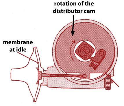
Once the membrane is fully expanded at high engine speed the shaft rotates the distributor base plate to achieve the maximum advance. Look carefully at the position of the cam in relation to the ignition points. This is exactly what you want to achieve, the ignition time is advanced when the engine runs faster.
