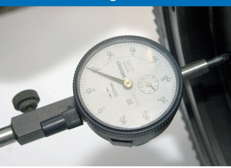
Once the dial indicator is installed against the flywheel, push the flywheel forward and position the dial gauge on the zero line (read your dial indicator manual to know how to do that). Then pull the flywheel and read the dial indicator. This is the crankshaft clearance or end play.
