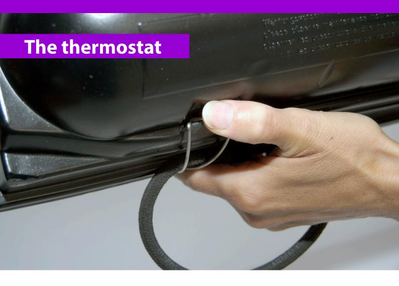
You need to open the air filter housing to access the thermostat. Unlock four metal clips to remove the air filter housing lid (as shown on the picture above). Remove the paper air filter to access the thermostat. You can replace the paper air filter if it is dirty, or use it again if it is a new one.
