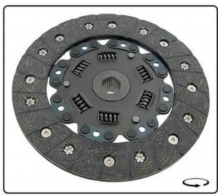
The clutch disc as shown on the picture above contains two friction plates, one on each side of the clutch disc, it is placed between the flywheel and the clutch pressure plate. The discs are composed from a series of slats secured with rivets. These slats are connected to the central hub using pressure springs. These springs are working just like your shock absorbers on your VW, they will absorb the vibrations caused by the engine.
