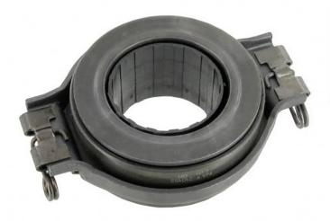
When you press the clutch pedal, the inner ring of the clutch release bearing will press against the clutch pressure plate. The outer ring stands still. This is possible because both rings on the release bearing are mounted on ball bearings.
