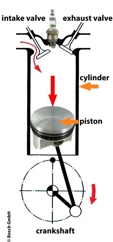
We show the first stroke on the drawing, the intake valve opens, the pistons moves towards the crankshaft, away from the spark plug, and sucks the air-fuel mixture coming from the carburetor (or fuel injector) into the cylinder. The valves are controlled by the camshaft and the push rods, we don't show them on this drawing to simplify. If you want to know more about this, read the article in edition 4 on page 42.
