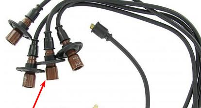
Some engines get interference from the spark plug cables, so you need to install spark plug cable with suppressors built in the heads (13, suppressor in the park plug heads). These suppres-
