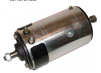
We show a 12 volts dynamo in the picture above. We don't need a rectifier in this case, the tension generated by the dynamo is already a direct current (or direct tension), ready to be used by our classic Volkswagen. The regulator will be found on top of the dynamo or under the back seat depending on the VW model.
